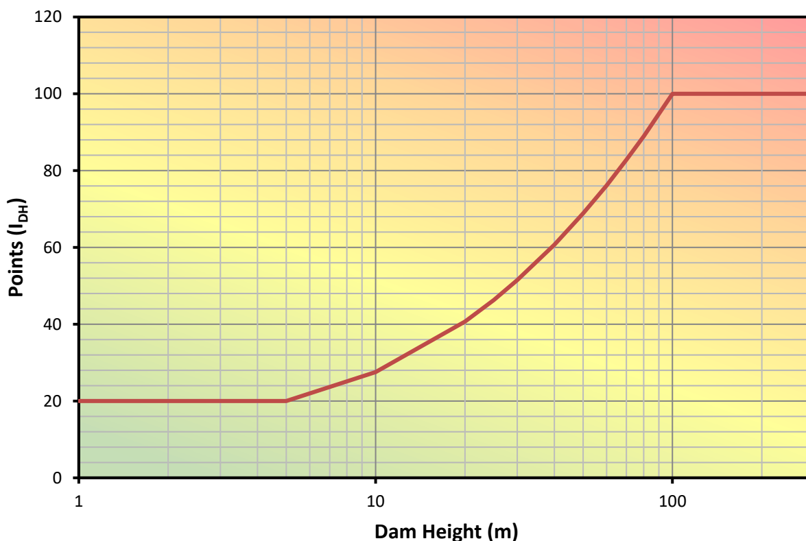
Figure 3.1.- Consequences Rating Points for Dam Height Index ( I_{DH} )
