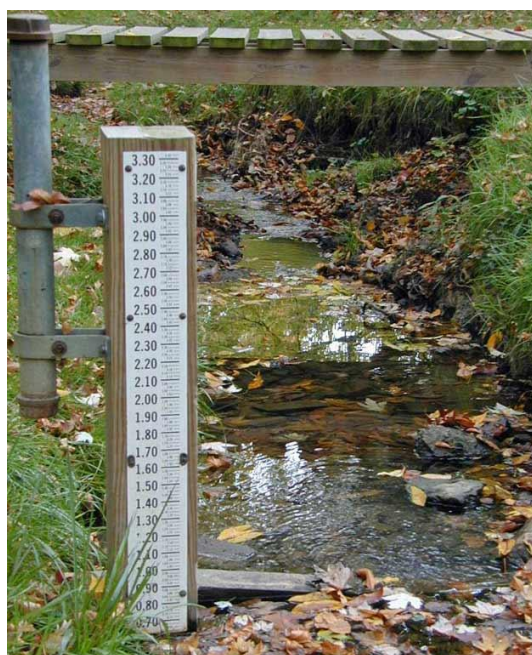
Figure 2-23. A staff gauge and crest-stage gauge installed next to a stream
