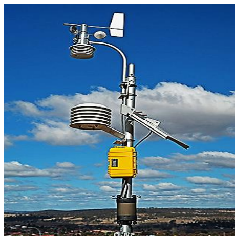
Figure 7-15. Automatic Weather Station
