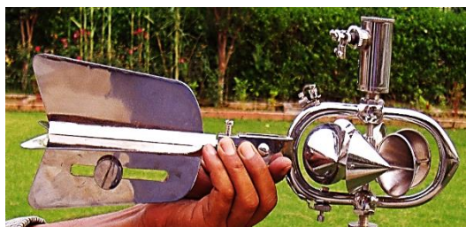
Figure 7-27. Vertical Axis Current Meter
