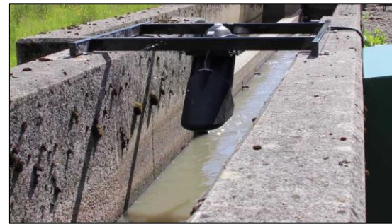
Figure 2-9. Laser-Doppler velocity meter with ultrasonic depth sensor measuring discharge in a drainage collection channel
