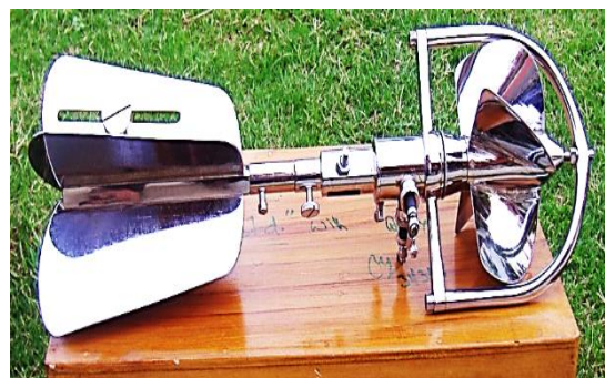
Figure 7-28. Horizontal Axis Current Meter
