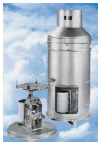
Figure 7-3. Weighing Type Rain Gauge
