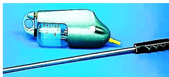
Figure 7-32. Depth Integrating Suspended Sediment Sampler
