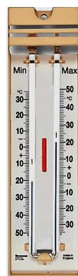
Figure 7-7. Maximum and Minimum Temperature Thermometer
