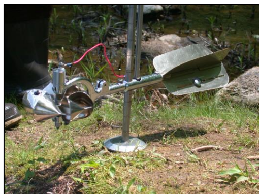
Figure 2-10. Standard propeller-type velocity meter
