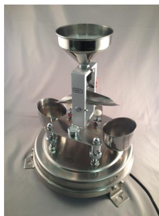
Figure 7-4. Tipping Bucket Recording Rain Gauge
