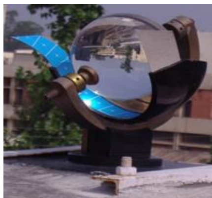
Figure 7-14. Campbell Stokes Sunshine Recorder
