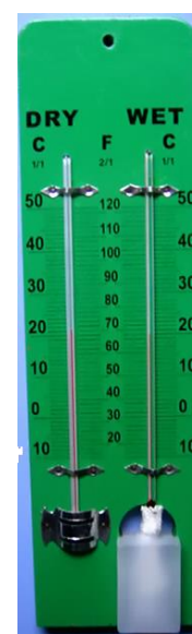
Figure 7-9. Dry and Wet Bulb Thermometer
