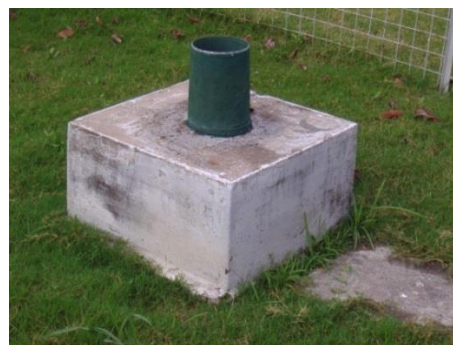
Figure 7-1. Indian Standard Ordinary Rain Gauge
