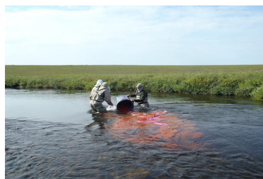
Figure 7-29. Dilution Technique of Velocity Measurement
