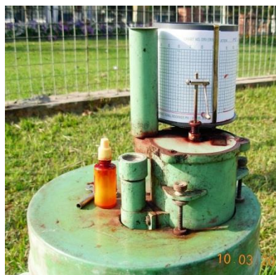
Figure 7-2. Indian Standard Natural Syphon Rain Gauge
