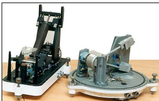
Figure 2-27. A long-period vertical seismometer (left) and a long-period horizontal seismometer (right)
