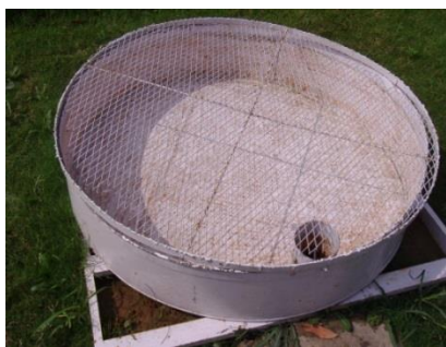
Figure 7-6. Indian Standard Evaporation Pan
