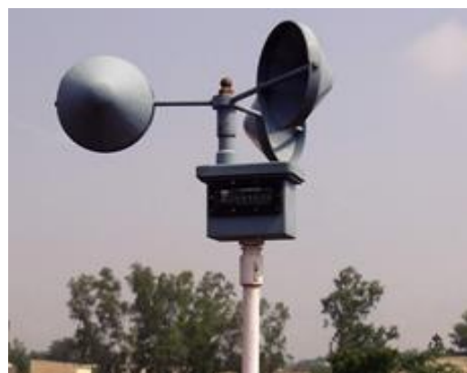
Figure 7-13. Cup Counter Anemometer
