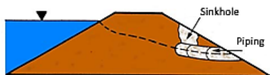
Figure 4-10. A sinkhole caused by a collapse into an animal burrow.
