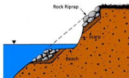
Figure 4-11. Wave action can remove riprap if it is not properly sized and installed. The illustration shows formation of a “beach” or bench and a subsequent scarp.
