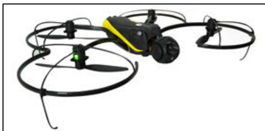
Figure 8-2. In the case of a four-propeller UAV system (quadcopter) such as the one shown, diagonal pairs of propellers spin in opposite directions
