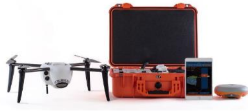
Figure 8-3. Rotary system drones suitable for dam inspection are small and easily transported.
