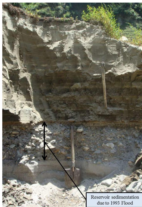
Figure 3-13. Sediment deposition strata in the Kulekhani reservoir in Nepal (a coarse layer deposition below in the layer appears to be deposited during 1993 floods) (Shrestha, 2012)
