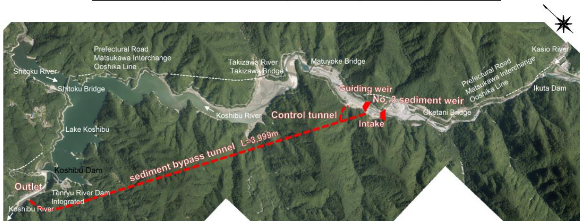
Overview of sediment bypass facilities
