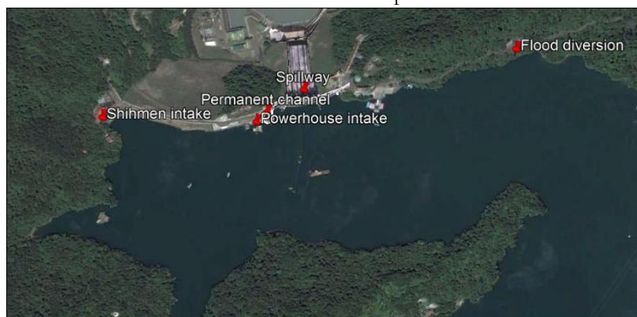
Figure 6-9. Location of existing outlets that may be used for sediment release (Google Earth image)
