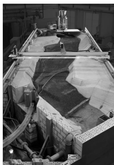
Figure 3-35. Physical model of sediment bypass at ETH-Zurich (Switzerland)
