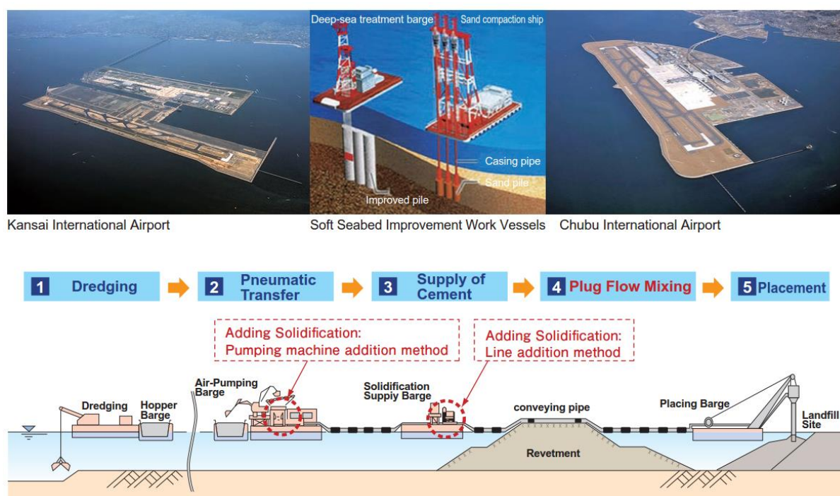
Figure 4-59. Some examples of artificial islands in Japan (upper pictures) and the workflow and features of dredged material recycling system ( www.umeshunkyo.or.jp/english/english.pdf )
