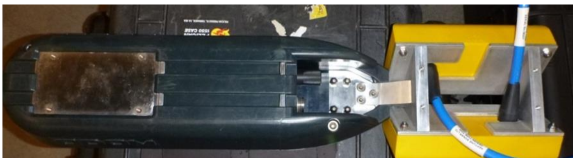
Figure A-6. Photograph of the system from the top which includes the Odom conventional multibeam transducer (left) and interferometric Bathyswath transducers (right). Motion compensation unit is located between the transducers ( Courtesy of USGS- Geomorphology & Sediment Transport Laboratory )
