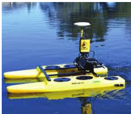
Figure 3-26. A surface drone, equipped with GPS, portable echo-sounder and other devices to measure bathymetry ( www.cansel.ca )
