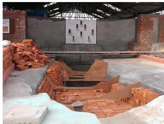
Figure 3-34. A physical model of a double arch dam in Hydro Lab (Nepal)
