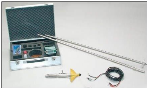
Figure 3-10. Current meter for flow measurement
