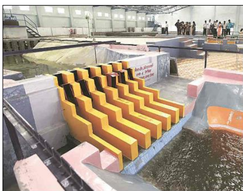
Figure 3-33. Physical model of a spillway at CWPRS (India)
