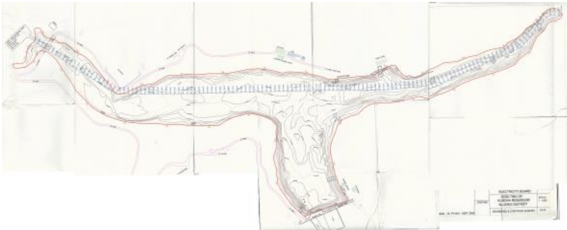
Example of bed topography of the Kundah forebay, measured in 2014
