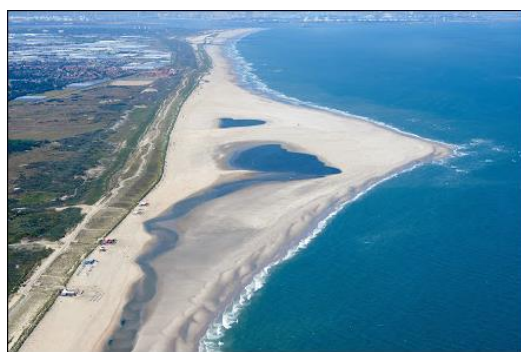
Figure 4-56. Sand nourishment along the coastline in North Sea ( www.dezandmotor.nl )
