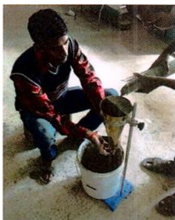
Figure 4-26: Flow-ability test by Marsh Cone apparatus in progress
