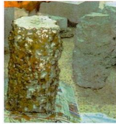
Figure 4-24: Chipped off Concrete Cylindrical Specimen
