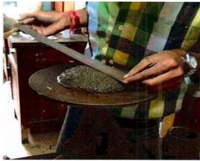
Figure 4-23: Flow-ability Test in Progress
