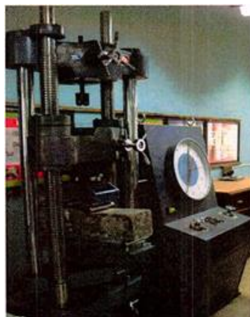
Figure 4-32: Flexure test setup for measuring toughness index
