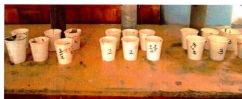
Figure 4-28: Gelification Test Set-Up
