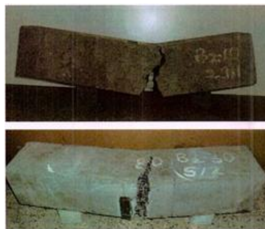
Figure 4-33: Toughness index tested beams
