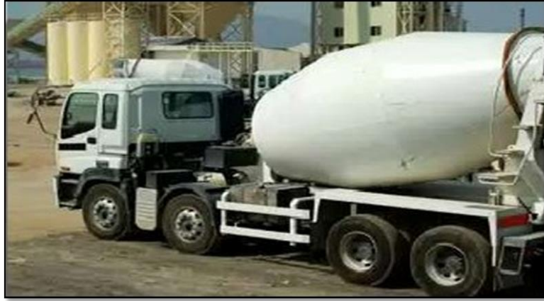
Photo 8: Transit mixer for transport of concrete
