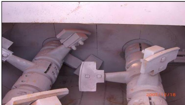
Photo 4: Paddles of Twin shaft mixer
