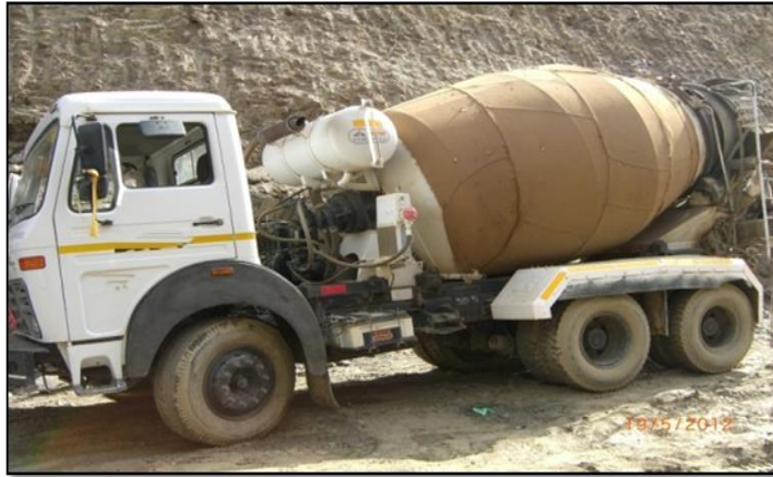
Photo 16: Temperature control- Wrapping the drum of Transit mixer by hazien cloth.
