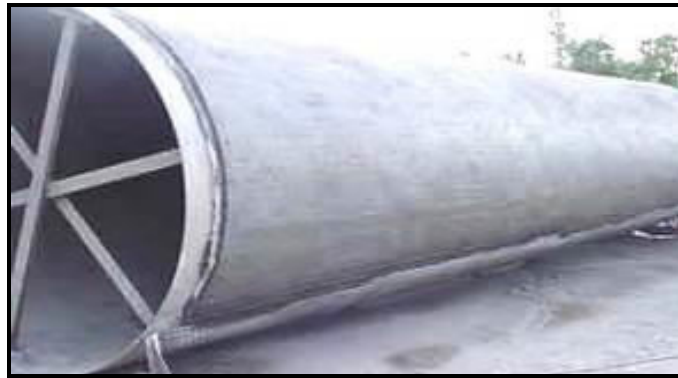
Fig 7.31 Outcoating of steel pipes
