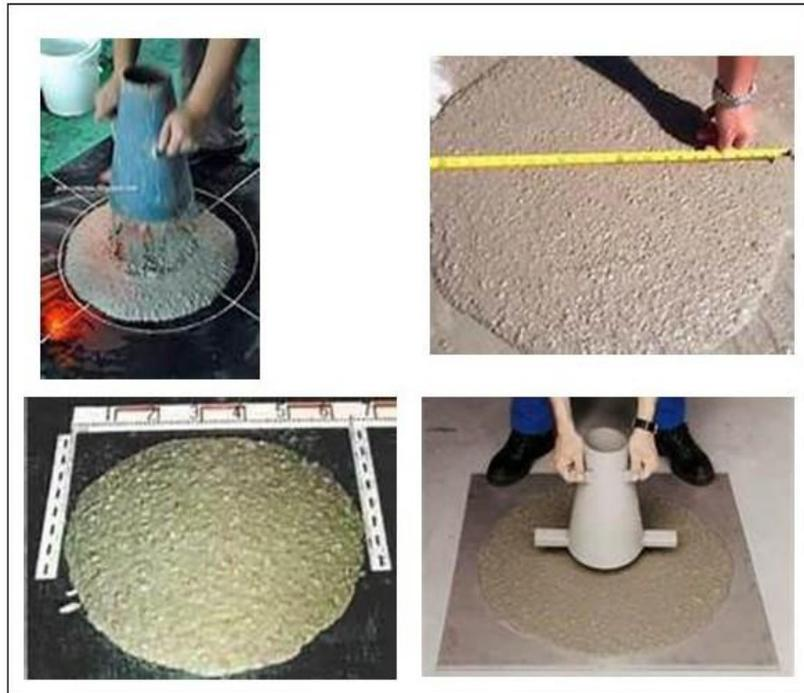
**Photograph 3. Slump-flow test**
