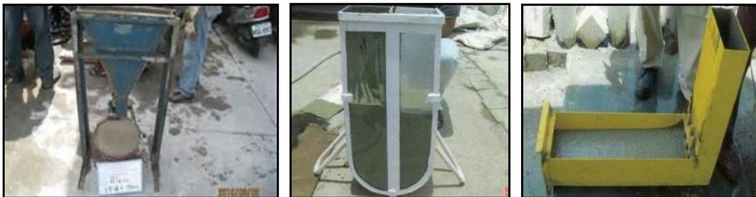
**Photograph 2. Test equipments: V-funnel, U-tube, L-box**
