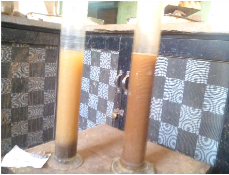
500 M.L. Capacity cylinder filling with below 75 Micron Hearting and Sand Sample
