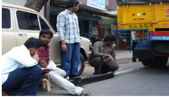
Photo: Testing of Rebound Deflection Using Benkelman Beam
