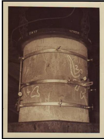
Photo no. 9: Arrangement for testing of Modulus of Elasticity on the core in laboratory.
