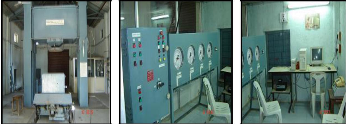
Photo no. 8: 2000 ton compression testing machine, control panel and computer system at M.E.R.I., Nashik
