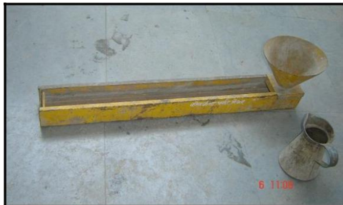
Photo no. 2 : Colgrout flow meter
